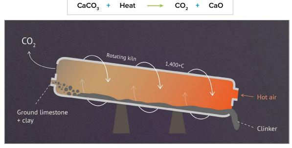
Cement and lime are manufactured in kilns according to the following reaction:
