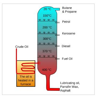
FIGURE 19: Overview of the Refinery Process | Source: CME Group
